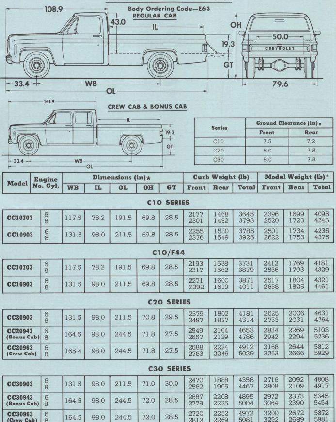
$<sup>\</sup>star$ Dimensions with standard equipment, unloaded. \*Model Weight includes Curb Weight plus occupants (standard seating capacity x 150 lb.). Total Model Weight may vary as much as  $\pm$  150 lbs. to allow for production build variation.
